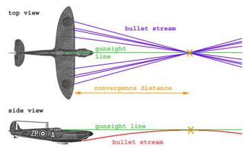
vertical as well as horizontal to adjust the bullet streams direction. Now all rounds meet (converge) in the orange X, a point at convergence distance on the gunsight line. The pilot can now use his pipper to aim. Also note that the rounds are now more concentrated on target, provided the pilot's shooting range is close to his set convergence distance.
